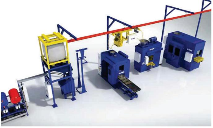
possible arrangement of a core sand processing and distribution system
