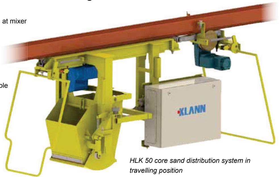
*HLK 50 core sand distribution system in travelling position*
